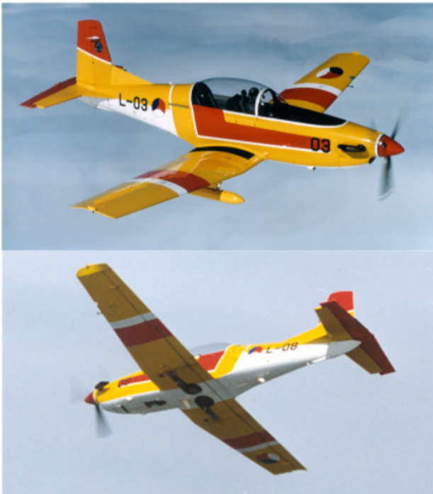
Figure 1. Photographs of the Pilatus PC-7. Length and wingspan are about 10 m. The current colour scheme is mainly yellow, red, white and black. When observed from a distance of 1 km, this aircraft subtends a visual angle of 1 degree (about the size of a thumbnail at arm's length). The black "nose" just in front of the cockpit prevents the pilot from being blinded by reflected sunlight.
