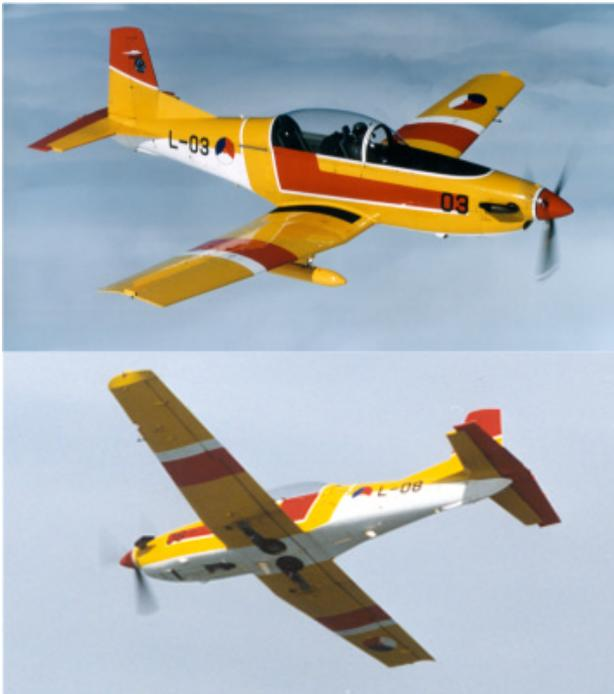
Figure 1. Photographs of the Pilatus PC-7. Length and wingspan are about 10 m. The current colour scheme is mainly yellow, red, white and black. When observed from a distance of 1 km, this aircraft subtends a visual angle of 1 degree (about the size of a thumbnail at arm's length). The black "nose" just in front of the cockpit prevents the pilot from being blinded by reflected sunlight.
