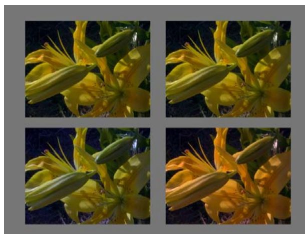
Figure 4. Screen layout of the visual experiment. The upper two images are identical references and represent the test scene under neutral D65 illumination. The lower two images correspond to the test scene rendered under one of the test illuminants (Red, Green, Yellow or Blue) after which a color constancy algorithm was applied. Different algorithms are used on the lower left and right image. Subjects had to indicate which of the two lower images had the best color reproduction compared to the upper reference images.
