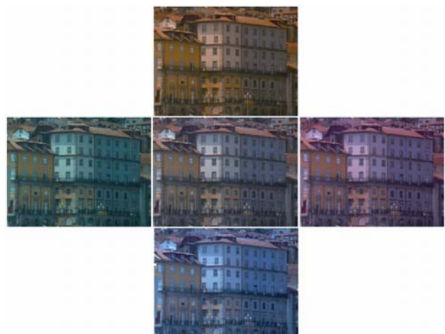
Figure 1. Scene 7 (one of our 8 test scenes) rendered under the different illuminants. The central image is under reference illuminant D65. Starting at the top position, in clockwise rotation the images correspond to the Yellow, Red, Blue and Green illuminant, respectively. The four chromatic illuminants are perceptually equidistant from D65, at 28 \Delta E_{ab} units. Prior to application of the spectral illuminants the calibration objects in the original images were removed, and resulting image gaps were filled in with the "inpainting" method of Criminisi et al. [9].
