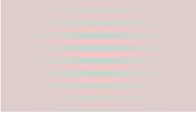
Figure 1: Stimulus example at high contrast for the 5700 K background in the Vogels & Lamboojij [1] study. Observers had to indicate perceived orientation of the stimulus which could be either horizontal or vertical.
