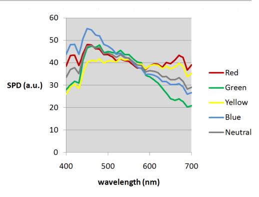
Distance to the neutral point was adjusted to obtain equal physical shifts in the reflected light signal when changing illumination from D65 to R,G,Y or B.
